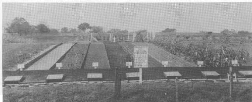
FIGURE 7.2 Site of the first plots in the United States for measuring runoff and erosion as influenced by different crops. The plots were established in 1917 at the University of Missouri. (Photograph courtesy Dr. C. M. Woodruff, University of Missouri.)
