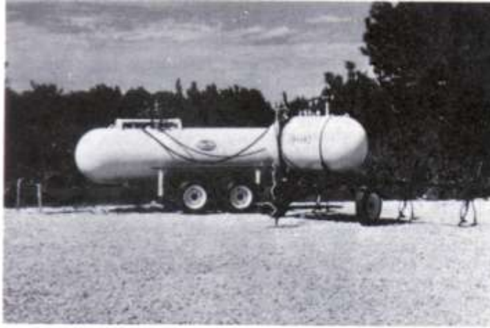
Figure 4. Transfer of Ammonia from Nurse Tank to Farmer's Applicator Using Vapor Transfer Pump.
