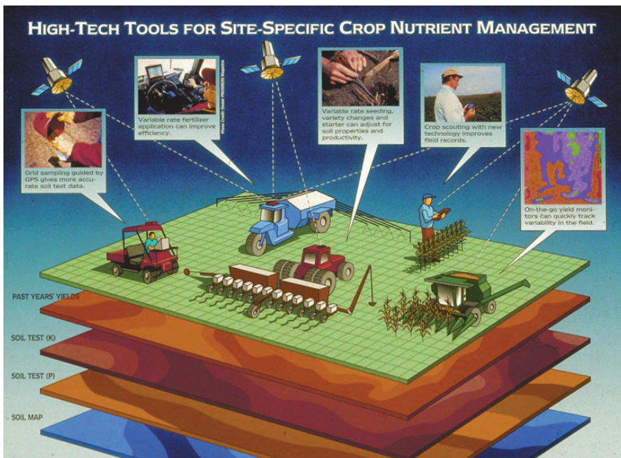
Figure 40. Illustration of various component practices and technologies commonly associated with specific precision agriculture systems (IPNI, Reetz, Better Crops, 1994).
