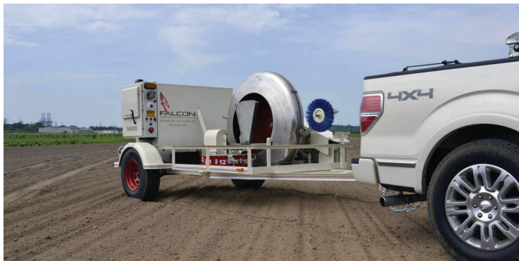
Figure 21. The Falcon automated soil sampling system included a stainless steel drum, with an attached soil probe, that collects samples as it rolls across the field, collecting samples, packaging, labeling, and cataloguing them, and transmitting sample site data to the internet “cloud” (Falcon Soil Technologies).
