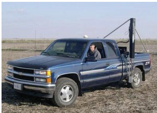
Figure 20. Hydraulic samplers mounted on a pickup truck or ATV help to reduce the workload in collecting soil samples, especially for deep sampling (CropSmith).
